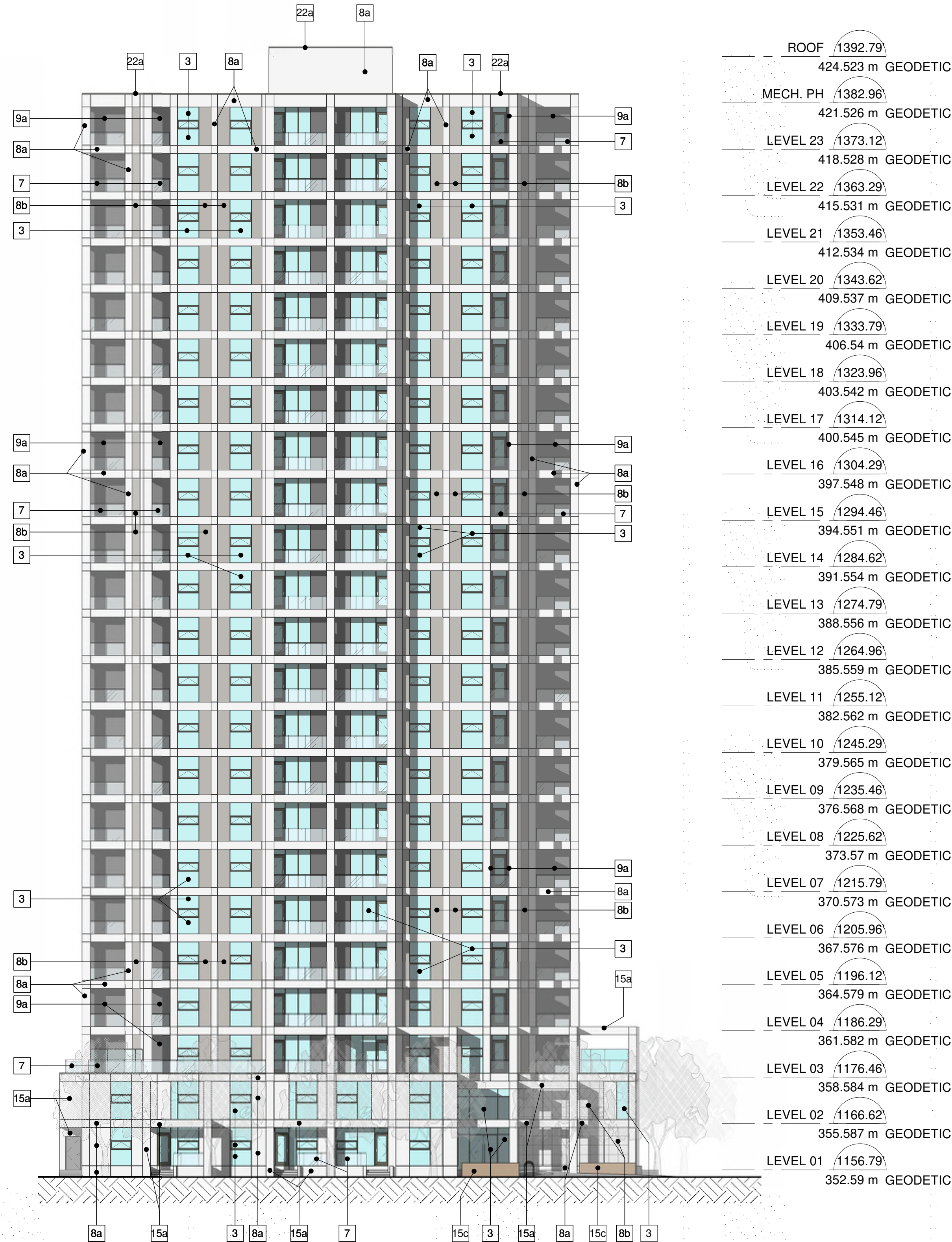
2 SOUTH ELEVATION DP2.03 SCALE: 1/16" = 1'-0"
